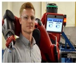
Collaborative robots or cobots are set to make working at production lines less taxing. They are to perform various tasks, such as helping employees to load machines and picking out device components from receptacles.
